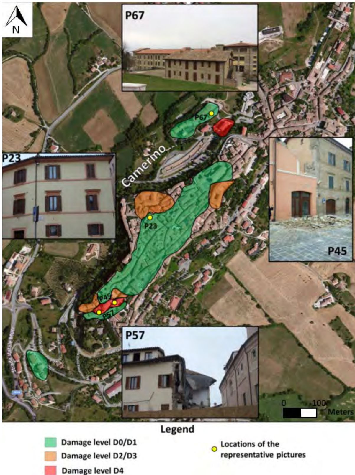
Figure 6. Damage zonation within the historic center of Camerino with pictures of the representative structures inspected.
