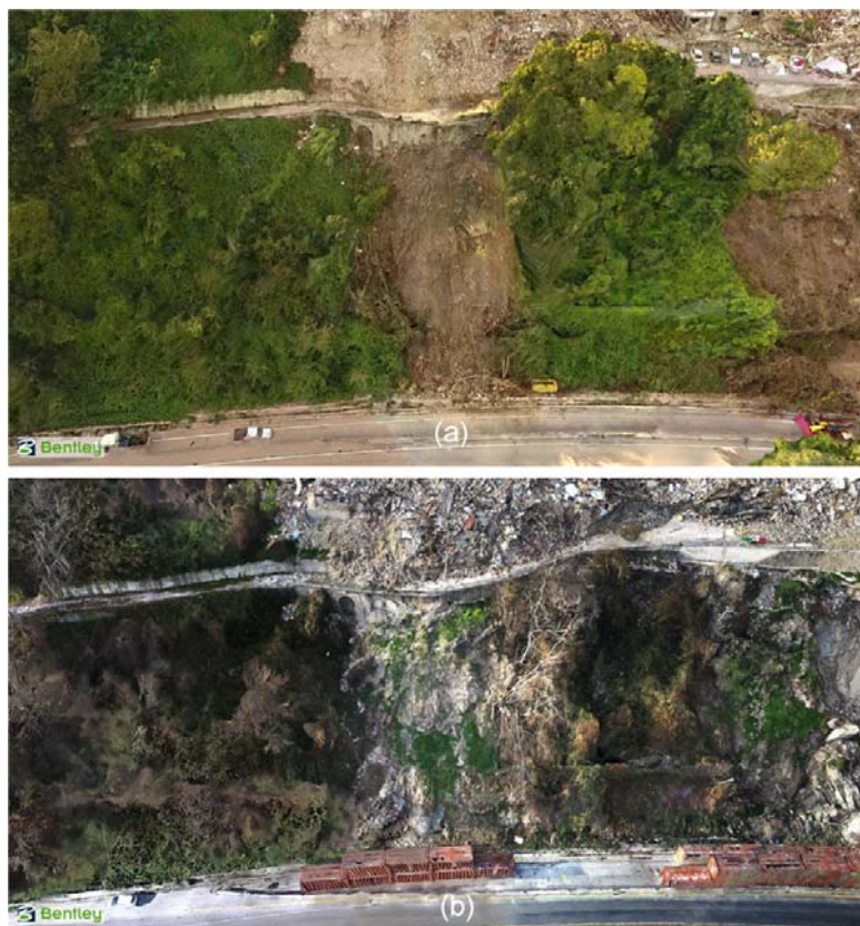
Figure 30: 3D model of the landslide #2 in Pescara del Tronto following: (a) the 24 August and (b) the 30 October event (from GEER, 2017).
