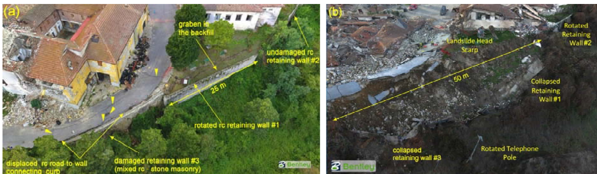
Figure 36: 3D model screenshots following: (a) the 24 August, and (b) 30 October event (from Lanzo et al., 2018).
