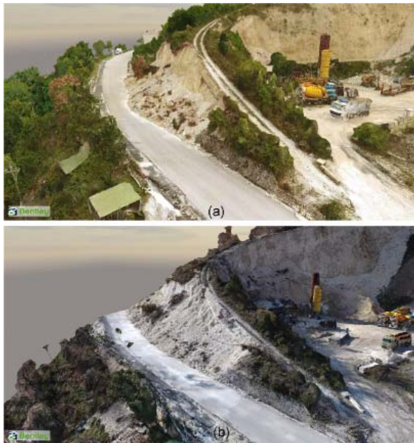
Figure 34: 3D model of landslide #7 and exposed pipeline following: (a) the 24 August and (b) the 30 October event (from GEER, 2017).
