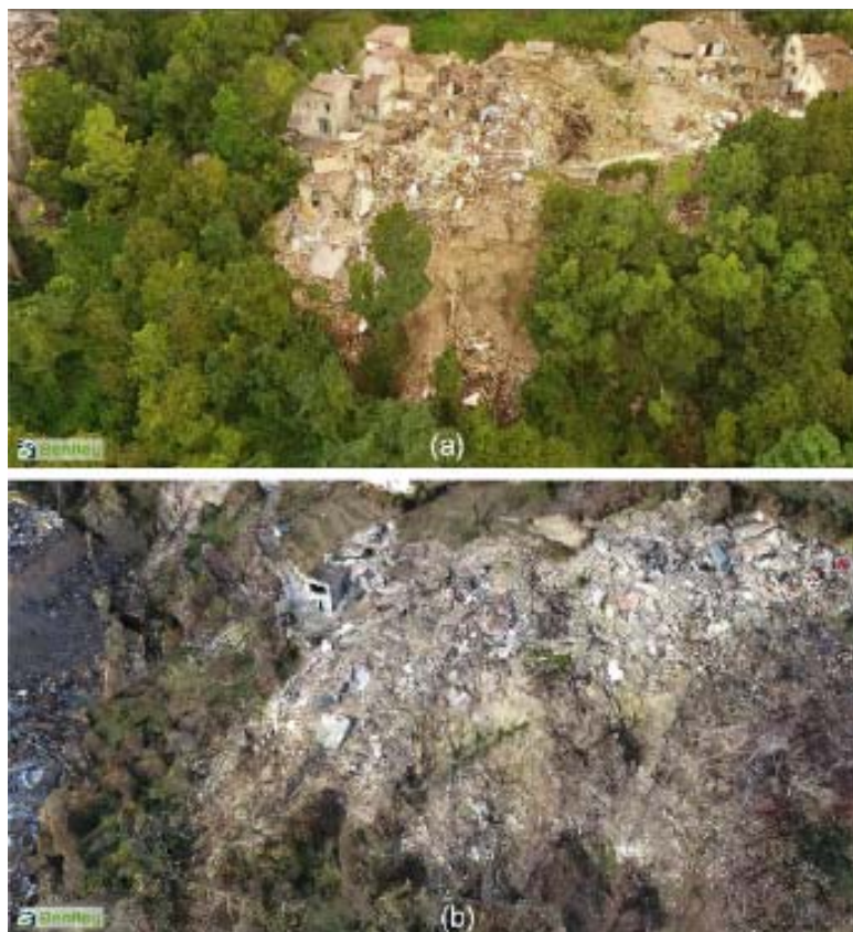
Figure 33: 3D model of landslide #6 following: (a) the 24 August and (b) the 30 October event (from GEER, 2017).
