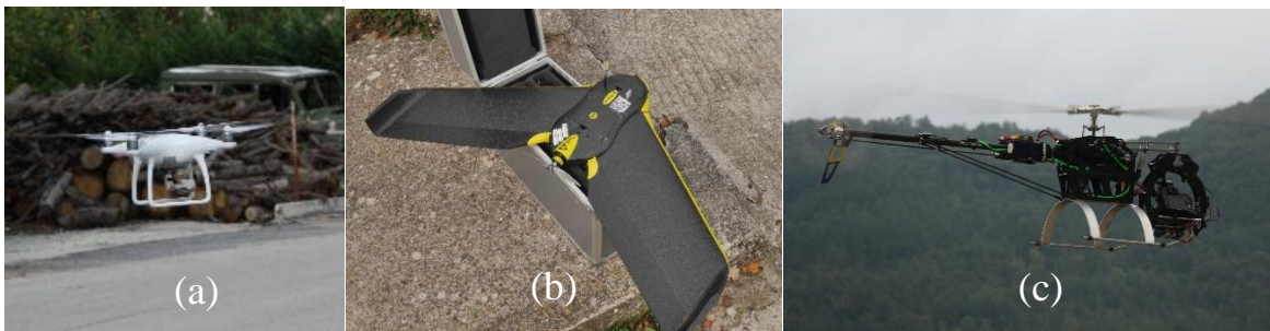
Figure 3. The employed UAV platforms in the Central Italy reconnaissance. (a) DJI Phantom 4, (b) Sensefly eBee, and (c) Align TRex 800e
