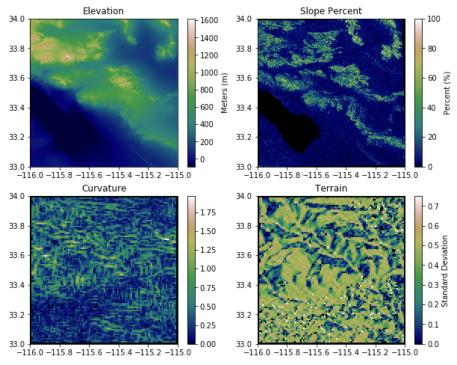
Elevation and slope plots from .tif file downloaded from USGS Earth Explorer at SRTM 1 Arc-Second Global in the Imperial Valley region of California
