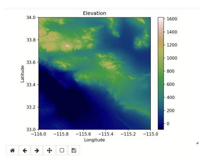
Interactive elevation and slope plots from .tif file downloaded from USGS Earth Explorer at SRTM 1 Arc-Second Global covering the Imperial Valley region of California
