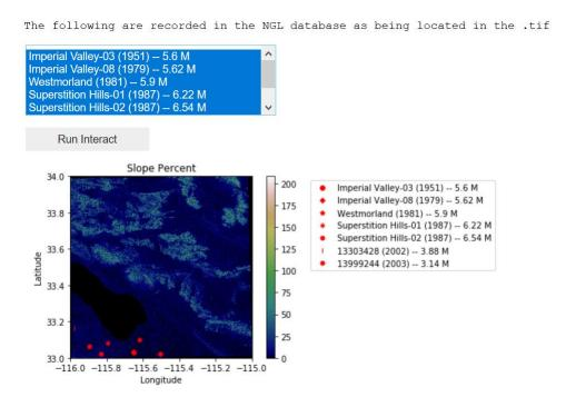
Slope plot from .tif file downloaded from USGS Earth Explorer at SRTM 1 Arc-Second Global containing events from the Imperial Valley
